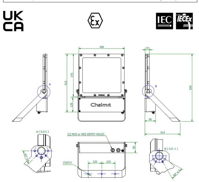
THE EVOLUTION X STIRRUP BRACKET HAS PRE-DEFINED FIXING ANGLES ALLOWING YOU TO AIM THE FLOODLIGHT AT INCREMENTS OF 30° OR 45° PLEASE REFER TO DIAGRAM ABOVE
